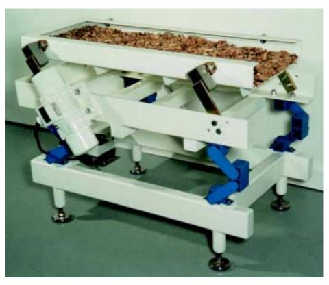
Demonstration conveyor trough for the ROSTA oscillating system "Silent Flow" with chassis excitation (energetic amplification). Oscillating trough suspended on 4 AU-DO 27 rocker arms, chassis suspended on 4 AB 27; driven by 2 unbalanced motors. Machine frame is installed on 4 mounts NOX 70, M16.
