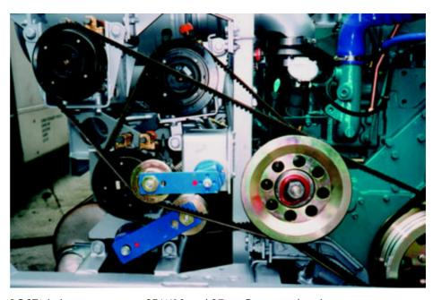
ROSTA belt tensioners type SE-W18 and 27 on Cummins diesel engine
