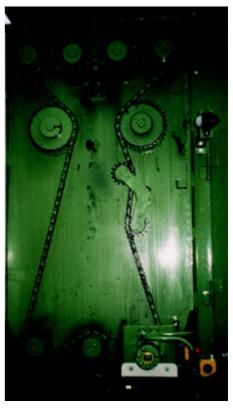
Tensioning of the chain drive system with SE-B 18 tensioner
