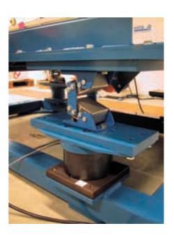
each case. Three-dimensional sensors (dynamic pressure transducers) are fitted underneath the ROSTA screen support, which precisely register the transmission of the reaction forces in the horizontal and vertical direction in continuous operation and when passing through resonance, which can then be visualised against a reference scale on a PC in a sinusoidal form, and can be printed out.
