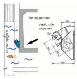
Guide roller for floating pontoon
