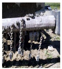
Rotary chain-roller drum for triggering mines
