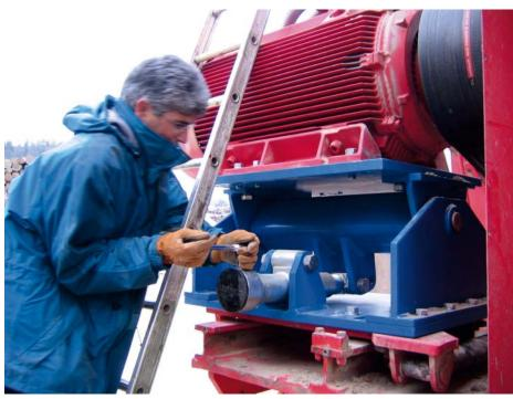
Tensioning the belt using a spindle gearbox
