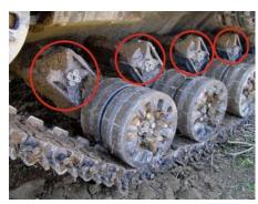
Elastic ROSTA suspension of the caterpillar guide rollers
