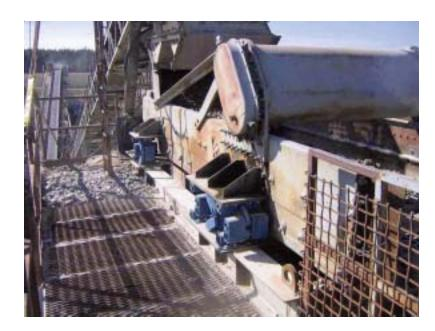
Fig. 1: Linear vibrating screening machine on ROSTA AB's in a very high steel-structure plant.
