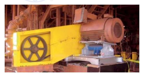
ROSTA motor base type MB 100 with 220 kW drive motor for a **Warman** centrifugal pump (Photo: BHP Billiton-Mining, Australia)
