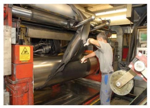
Once this process has been completed, the finished mixtures are stored for some time in the stacker for structure stabilisation, until they are ready for despatch or are transferred to the in-house extrusion and the subsequent vulcanisation processes.
