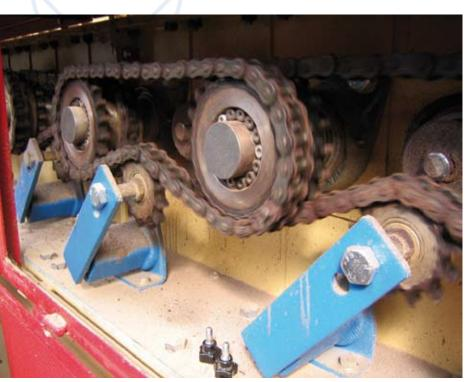
Elastic chain tensioners on an infeed section
