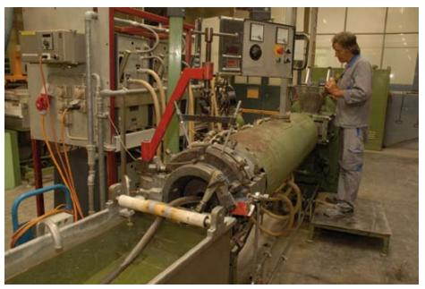
Extrusion of the ROSTA rubber profiles
