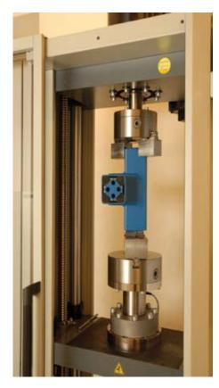
Torque testing machine in the ROSTA laboratory
