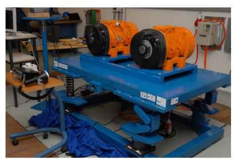
A laboratory trial was also set up for the "disbelievers" among the participants, which confirmed the 98.5% isolation effect. In addition, a comparative measurement of the "ROSTA ABs: Helical springs" residual force transmission was also carried out on this test bench.
