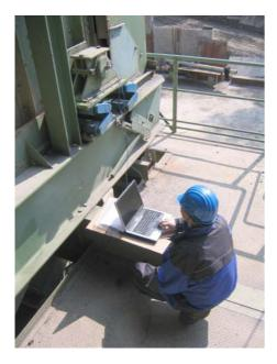
Even the measurement of the isolation efficiency was not forgotten! Do the ROSTA oscillating mountings really dissipate 98% of the vibrations? Yes, as much as 98.5% is "swallowed up" here by the ABs.
