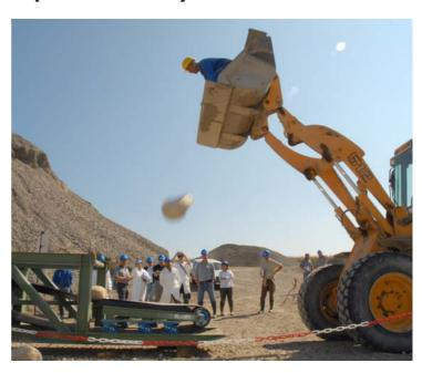
Not all the sales technicians were convinced of the efficiency of the ROSTA Impact Table at the transfer stations. The sharp-edged 100 kg chunks falling from a height of 5 metres should prove the effectiveness of the ESL anti-vibration mountings. After thirty drops = not the slightest injury to the conveyor belt!
