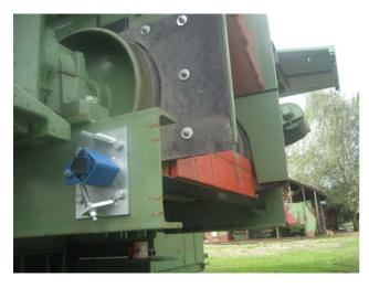
Demonstration of the new development of a self-adjusting ROSTA suspension system for the so-called drumhead scrapers. The Type DR 38 x 80 rubber suspension units that are fixed on both sides of the rubber belt frame can be synchronously pre-tensioned thanks to the tension scale and thereby provide an identical compression over the complete width of the belt.
