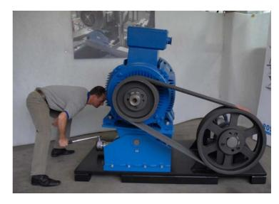
Pretensioning of the 250 kW belt drive using a simple ratchet lever. The extremely light running bevel gear lifting spindle makes the easy handling of the ROSTA Type MB 100 motor drive possible without additional aids such as hydraulic cylinders, etc. The radial tensioning force required here for the six SPC drive-belts was 17,992 N!
