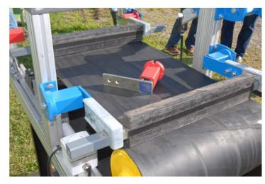
Suspension of crossover scrapers with ROSTA Type SE tensioning elements and, in comparison to the indefinable copy-tensioners that already "run-out" in practical trials after five minutes and no longer press the cleaning strips onto the belt.
