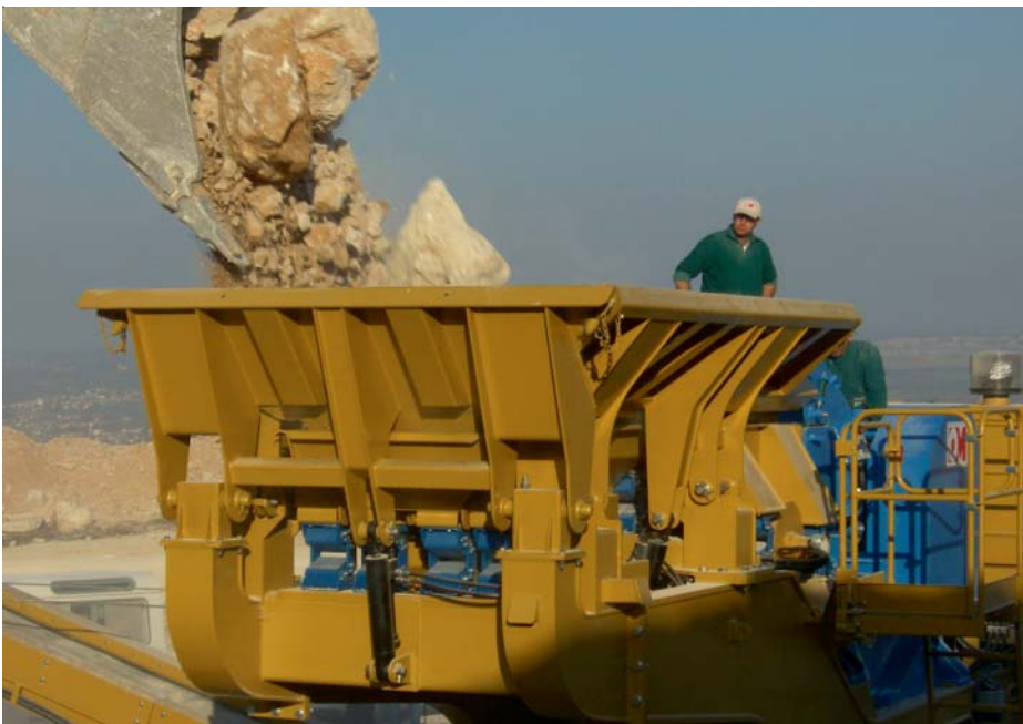
Feeding chute for mobile crusher mounted on AB-D 50-2
