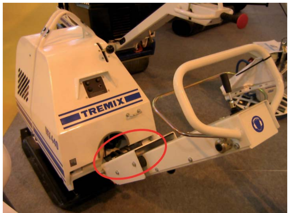
Flexible suspension of the compactor operating console
