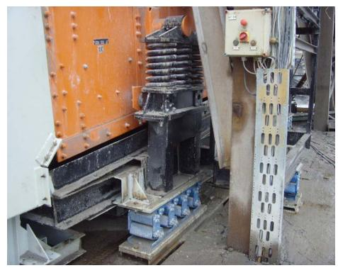
LZG screen with helical spring suspension, and the counterframe supported on 14
