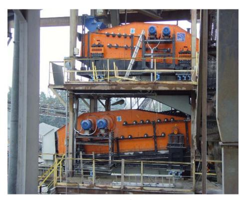
Two LZG linear vibratory screens on a counterframe with successive grain size selection (large grain outflow = upper screen; fine grain outflow = lower screen)
