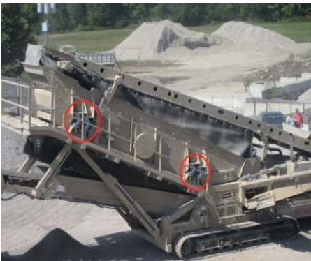
ASTEC Type 2516 T screen, with belt loading, suspended on 8 pcs. ROSTA AB-HD 50-2 elements
