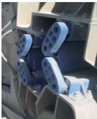
Screen suspension on the feed-end side using two AB-HD 50-2 by the maximum inclination angle of 25°
