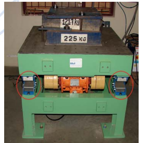
Accumulator test-bench mounted on 4 ROSTA oscillating mounts type AB-D 27
