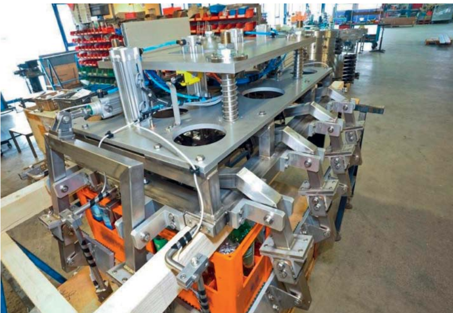
WYSS gripper head with 12 clamping claws
