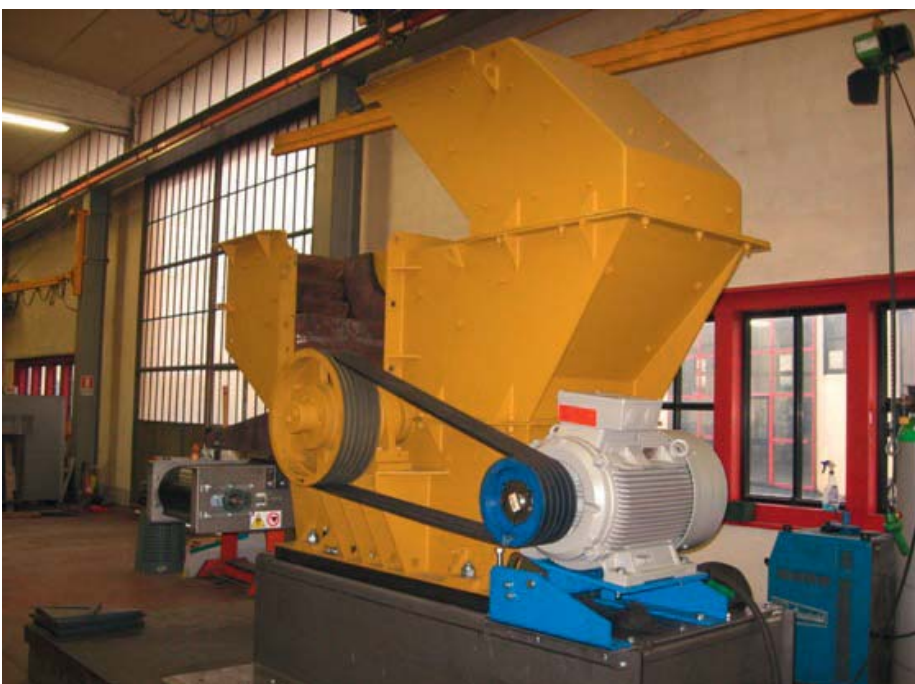
Centrifugal crusher 45 kW, 225 M with 5-strand SPB belt set, ROSTA MB 50 x 500
