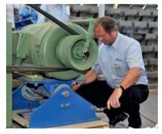
The "older and wiser heads" immediately understood the handling advantages of the new horizontal pre-tensioning device with prapezoidal screws on the MB 70
