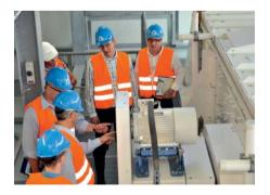
Elliptical screen drive suspended on motorbase type MB 50 x 270-2, does the positioning correspond to the direction of drive rotation?
