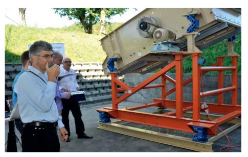
Counter-mass frame (red) positioned on oscillating elements type AB-D 50
