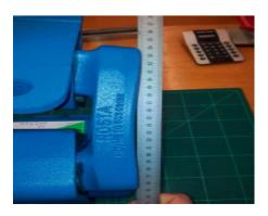
Test unit HS 50 after 10 times overload = slight deformation of the arms
