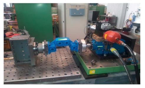
Testing device for swinging (dynamic) stress at EMPA
