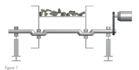
of the springs is a must, as it is the springs and not the bearings that bear the main load of the screen box.
